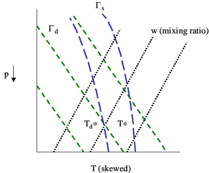
Knowing  $T$  and  $p$  (point  $T$  on the diagram) the mixing ratio lines can be interpolated to give the saturation mixing ratio - the amount of vapor the air can hold in g/kg at saturation.
