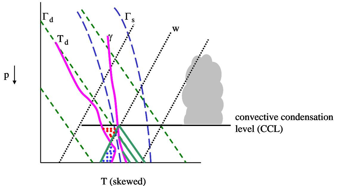
The solid line (labeled  $\gamma$ ) is the original sounding, say, at sunrise. Solar heating progressively heats the surface and warms the lowest layer of air. The convective mixing generates a layer of constant potential temperature and constant mixing ratio until, eventually, the air is saturated at the top.
