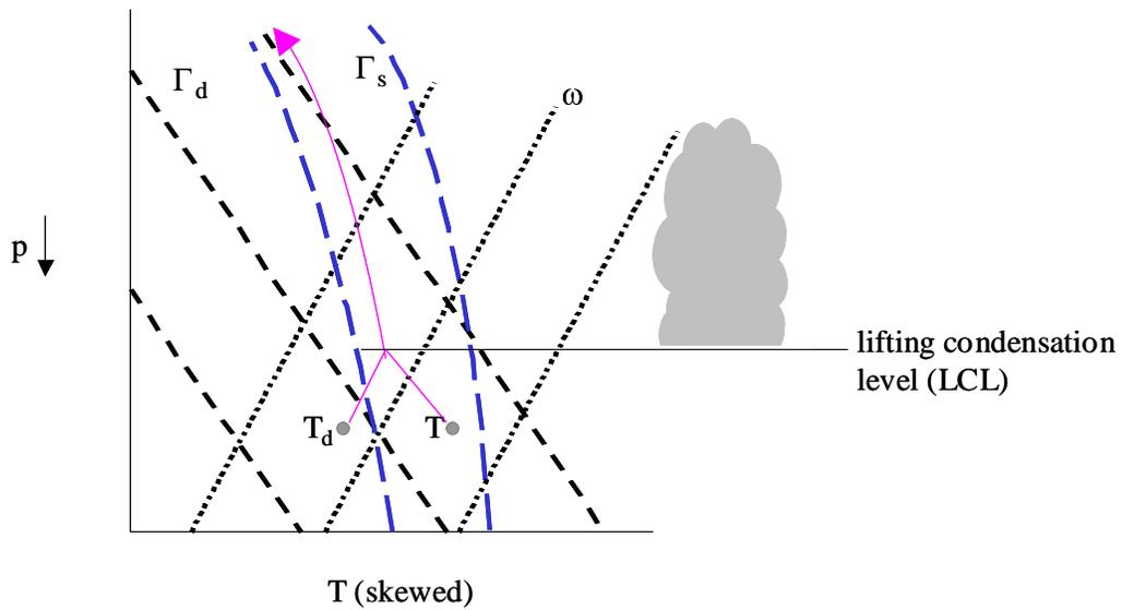
The lifting condensation level is the level at which  $T$  reaches  $T_d$  (which itself has decreases but at a lesser rate). The air is now saturated and continued lifting causes condensation in the form of a cloud. Above the LCL, a parcel of air will follow the saturation adiabat.
