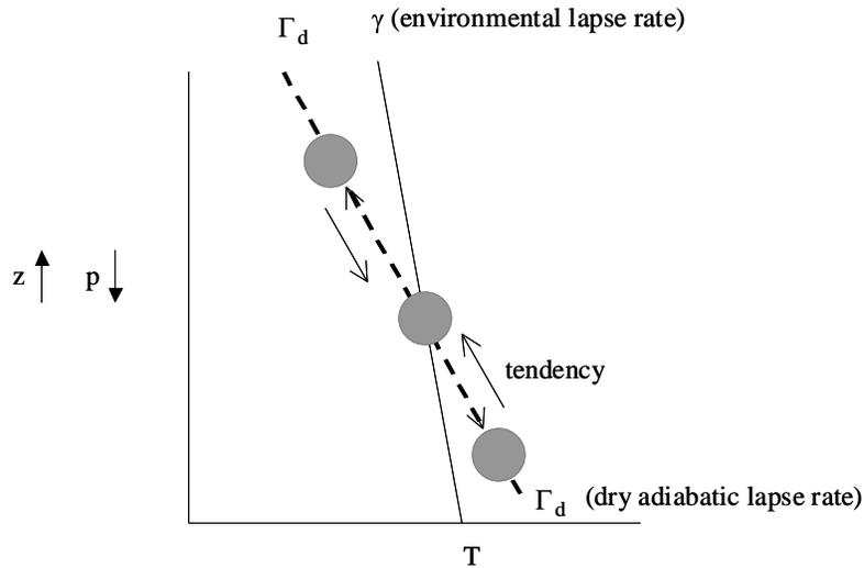
Consider a parcel at a given pressure level. Impose a displacement in the vertical direction (upward or downward).
