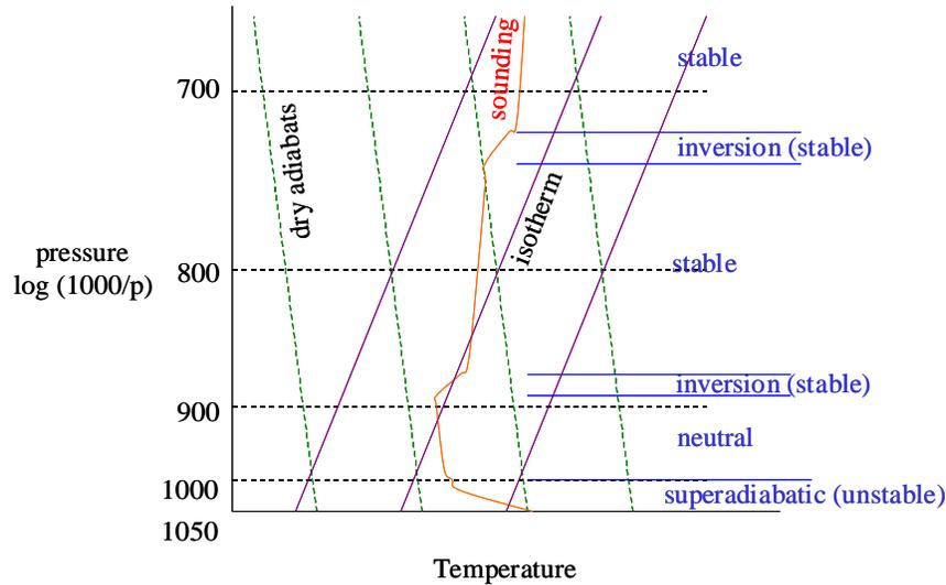
**Note:** some of these layers may be "conditionally stable" depending on whether the air is saturated with moisture.
