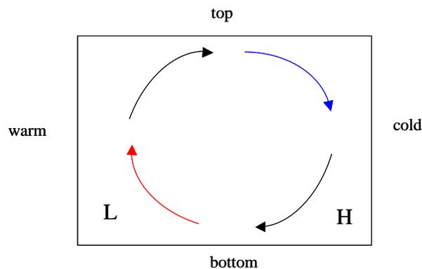
The buoyant rise of the fluid along the heated side creates a decreased pressure (L) at the lower left corner, while the negative buoyancy at the cold side produces a higher pressure (H). This pressure difference drives the fluid across the lower surface of the container. Based on such a thermally driven circulation, one can image a similar pattern of air motion within the atmosphere as a consequence of differential heating.
