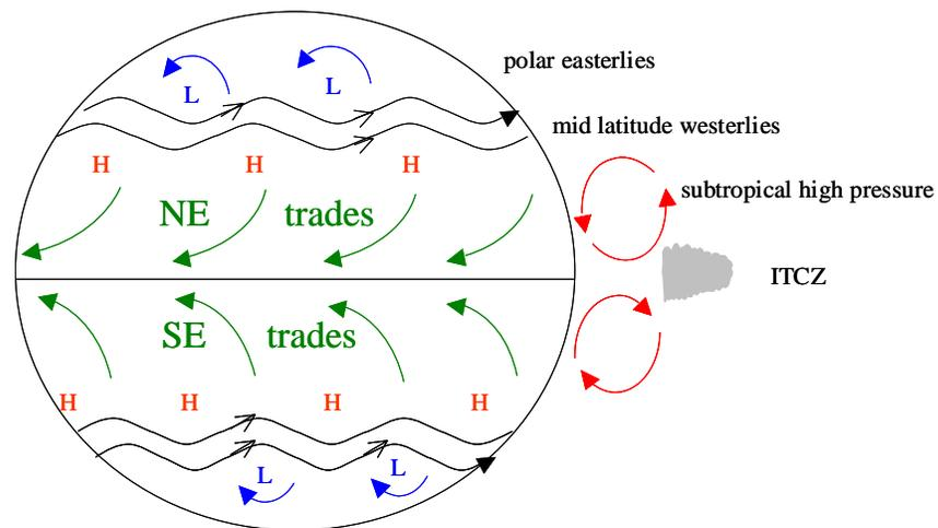
Where the N-hemisphere and S-hemisphere Hadley cells come together, there is convergence in the low level winds. The predominant rising motion results in a band of extensive convective clouds and high rainfall. This band is often shown by satellite photographs to be continuous for many thousands of kilometers but the influence of continents and large ocean bodies perturb the pattern shifting the convergence zone north or south, and making it discontinuous.
