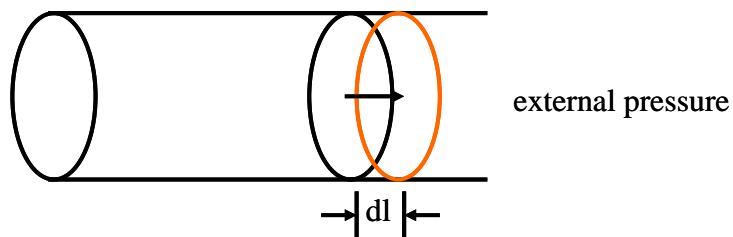
Let the cylinder contain unit mass of air (1 kg). The work done in the expansion is equal to the force ( $pA$ ) multiplied by the distance moved by the cylinder  $dl$ .
