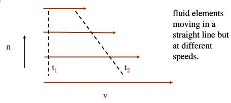
Consider a marker in the fluid such as the dashed line crossing the streamlines. Initially, the marker might be normal to the streamlines, as at time  $t_1$ , but later will be rotated to the position at  $t_2$ . The marker line has undergone an anticlockwise rotation (cyclonic in the N-hemisphere). We evaluate the contribution to the
