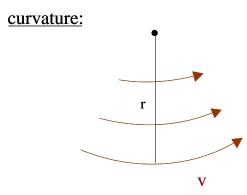
If, at radial distance r, the velocity is V, the curvative component of vorticity is evaluated as V/r in
